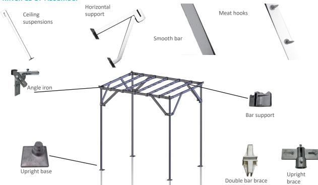
For spans in excess of 2 m, the rack is reinforced by two intermediary uprights (with the two accessories opposite : upright brace, double bar brace).
